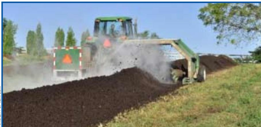
Here, a tractor turns the windrow composting pile on the farm used in the study.
